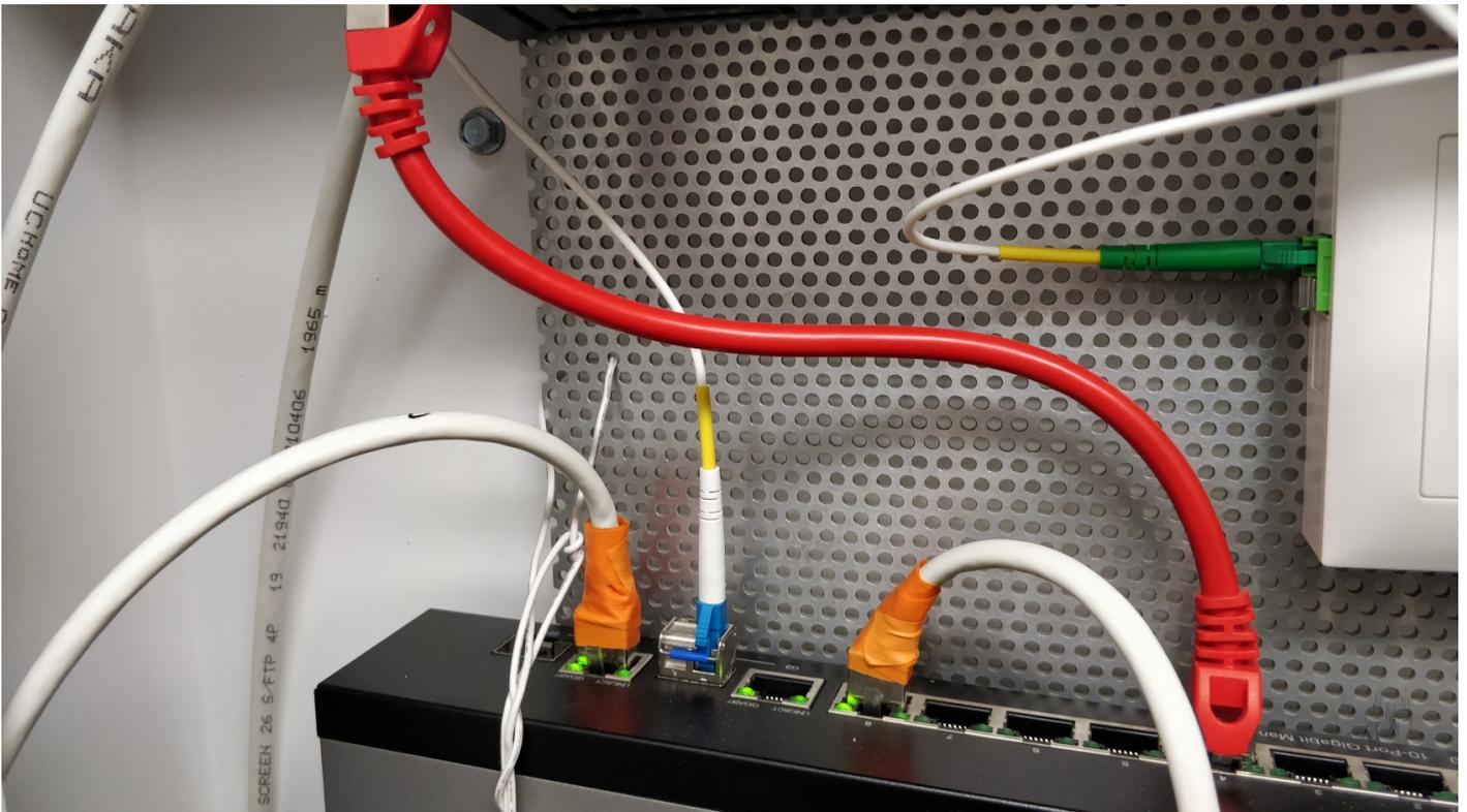
The setup is refreshingly simple, I added an SFP modul (FLEXOPTIX S.B1312.10.XDL) to the Cisco SG300-10 switch I used before, that was all. With my new provider [iWay](#) it was not even necessary to configure a specific VLAN.
