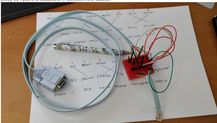
To connect the wires to the breadboard I did crimp connectors to them.
